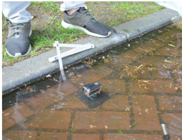
Figure 6. Minidiver installed; hand measurement point; underwater camera set-up.
