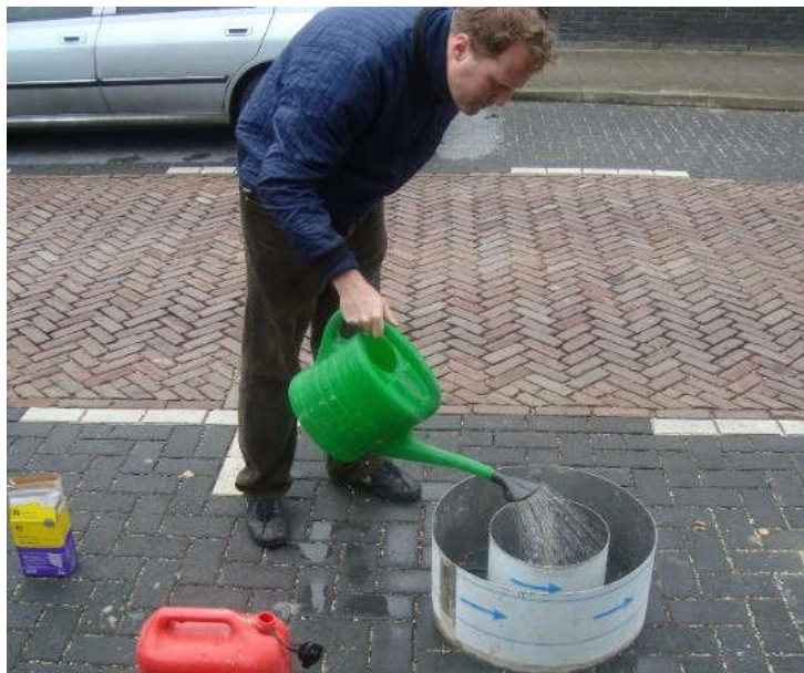
Figure 4. Double-ring infiltrometer tests.
